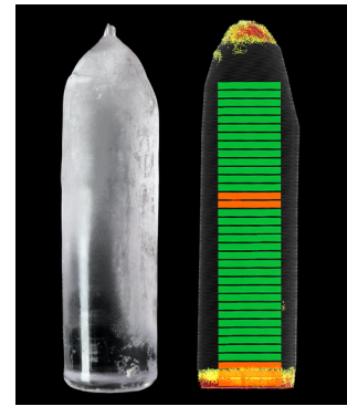
Figure 7. Verneuil-grown sapphire crystal (left) and its digital twin with defect pattern and wafering plan (right). The extraction yield (green: defect-free préparages) is 33.6%.
