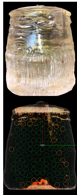
Figure 8. 260 kg KY sapphire (top) and its digital twin with defect pattern and coring plan. Green – defect-free cores; yellow – partly defective ones. The extraction yield is 31%.
