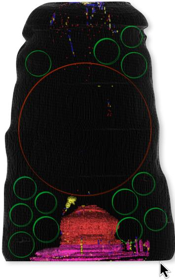
Operator can rotate 3D model, measure defects and optimise coring.
