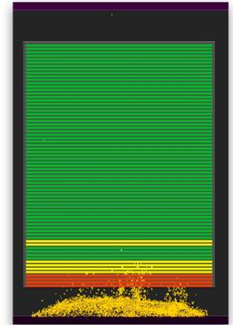
Figure 6: Wafer compliance in the crystal 3121-4. Green - good wafers, yellow - defects detected by TotalScan™ in raw crystal, red - defects detected by TotalScan™ in raw crystal and Candela® in wafers.
